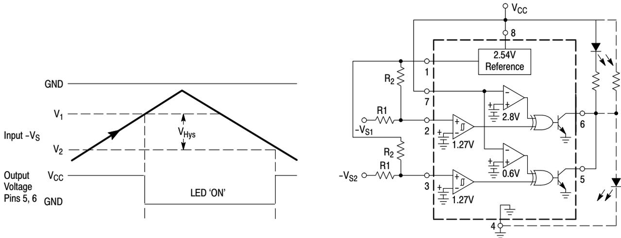
The above figure shows the MC34161 configured as a dual negative undervoltage detector. As the input voltage decreases towards ground, the LED will turn 'ON' when  $-V_{S1}$  or  $-V_{S2}$  falls below  $V_1$ . With the dashed line output connection, the circuit becomes a dual negative overvoltage detector. As the input voltage increases from ground, the LED will turn 'ON' when  $-V_{S1}$  or  $-V_{S2}$  exceeds  $V_2$ .
