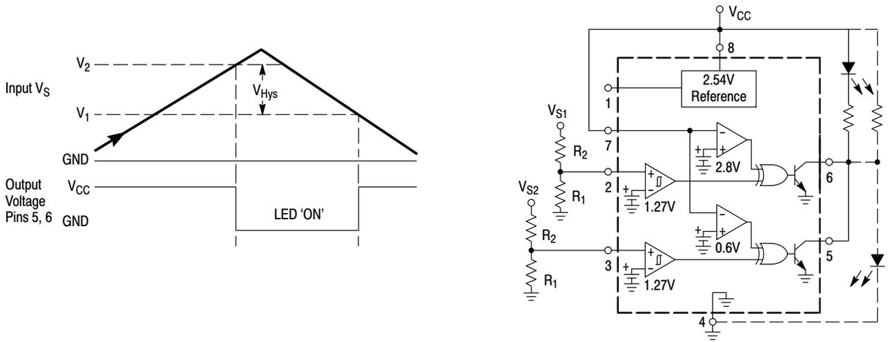
The above figure shows the MC34161 configured as a dual positive overvoltage detector. As the input voltage increases from ground, the LED will turn 'ON' when  $V_{S1}$  or  $V_{S2}$  exceeds  $V_2$ . With the dashed line output connection, the circuit becomes a dual positive undervoltage detector. As the input voltage decreases from the peak towards ground, the LED will turn 'ON' when  $V_{S1}$  or  $V_{S2}$  falls below  $V_1$ .
