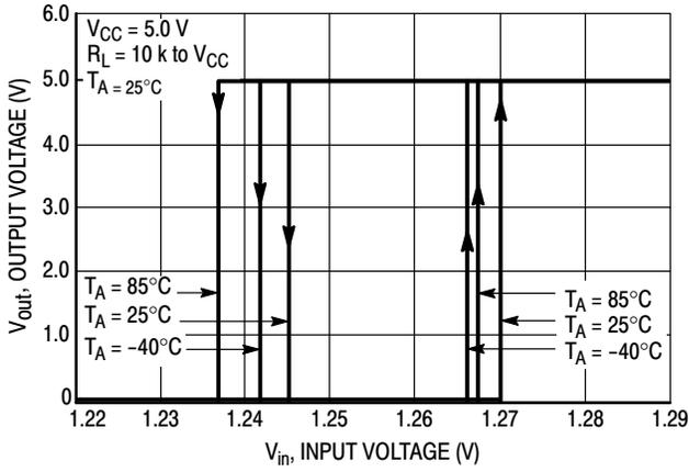
Figure 2. Comparator Input Threshold Voltage
