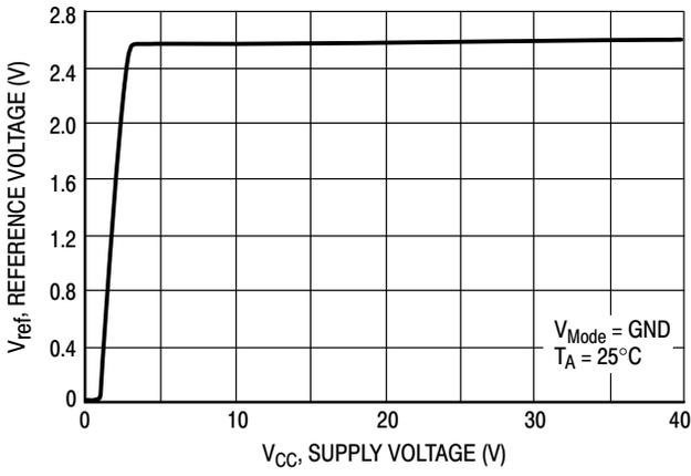
Figure 8. Reference Voltage versus Supply Voltage
