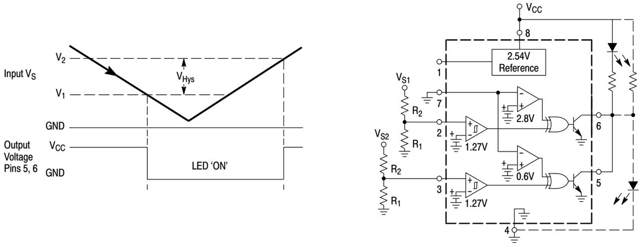
The above figure shows the MC34161 configured as a dual positive undervoltage detector. As the input voltage decreases towards ground, the LED will turn 'ON' when  $V_{S1}$  or  $V_{S2}$  falls below  $V_1$ . With the dashed line output connection, the circuit becomes a dual positive overvoltage detector. As the input voltage increases from ground, the LED will turn 'ON' when  $V_{S1}$  or  $V_{S2}$  exceeds  $V_2$ .
