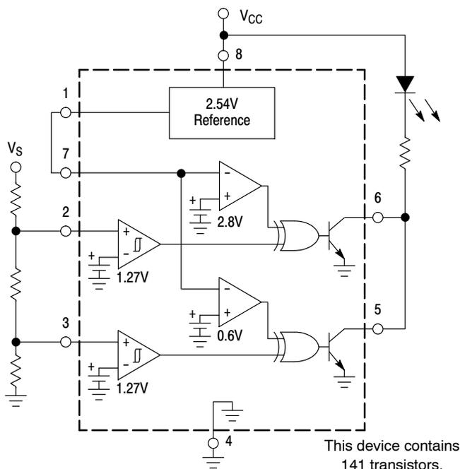
**Figure 1. Simplified Block Diagram**
