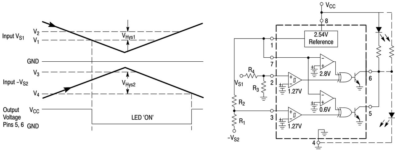
The above figure shows the MC34161 configured as a positive and negative undervoltage detector. As the input voltage decreases toward ground, the LED will turn 'ON' when either  $V_{S1}$  falls below  $V_1$ , or  $-V_{S2}$  falls below  $V_3$ . With the dashed line output connection, the circuit becomes a positive and negative overvoltage detector. As the input voltage increases from the ground, the LED will turn 'ON' when either  $V_{S1}$  exceeds  $V_2$ , or  $-V_{S1}$  exceeds  $V_1$ .
